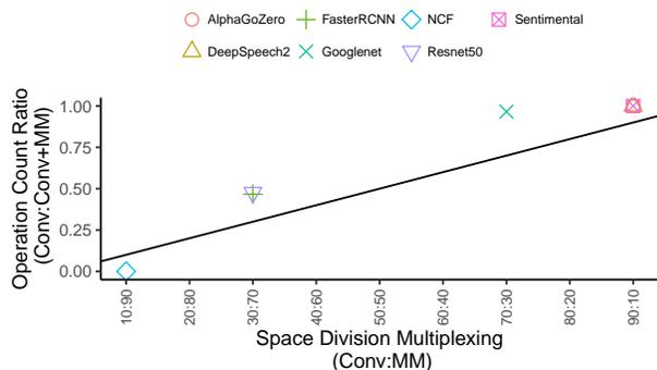
Fig. 11: Correlating MLPerf benchmark characteristics to Space Division Multiplexing arrangement.
