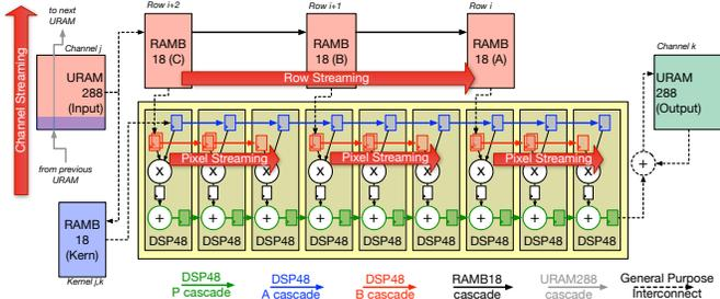
(a) Design of a  $3 \times 3$  convolution block. DSPs configured in SIMD=2 mode, a set of 8b weights are shifted into the *B* cascade. One stream of  $2 \times 8b = 16b$  data streamed into the *A* cascade from different rows. BRAM cascades also configured to exploit row reuse.
