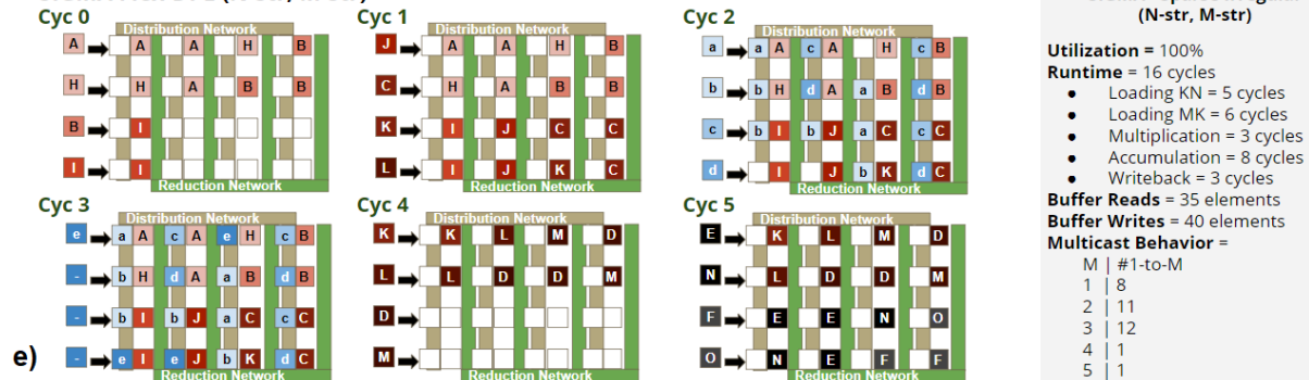
Figure 4: (a) Example GEMM matrices. (b) Mapping comparison between systolic array and SIGMA Flex-DPE for dense regular GEMMs. (c) Dense irregular GEMMs comparison. (d) Sparse irregular GEMMs comparison. (e) Alternative sparse irregular Flex-DPE mapping. (Note: M-str means MK matrix is streaming, N-sta, means KN matrix is stationary, etc.)
